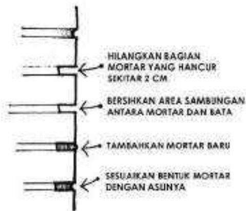
Gambar II. 2 Cara melakukan Repointing
